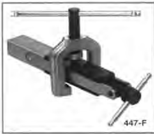
Feed release and burnishing mechanism.
